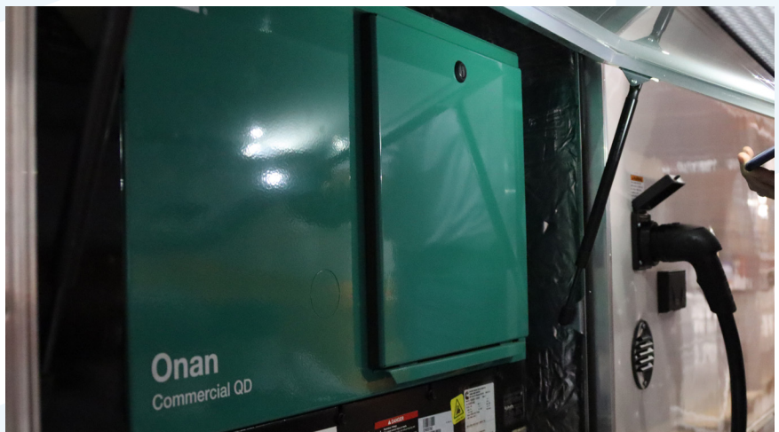
Commercial grade Cummins® ONAN generator
